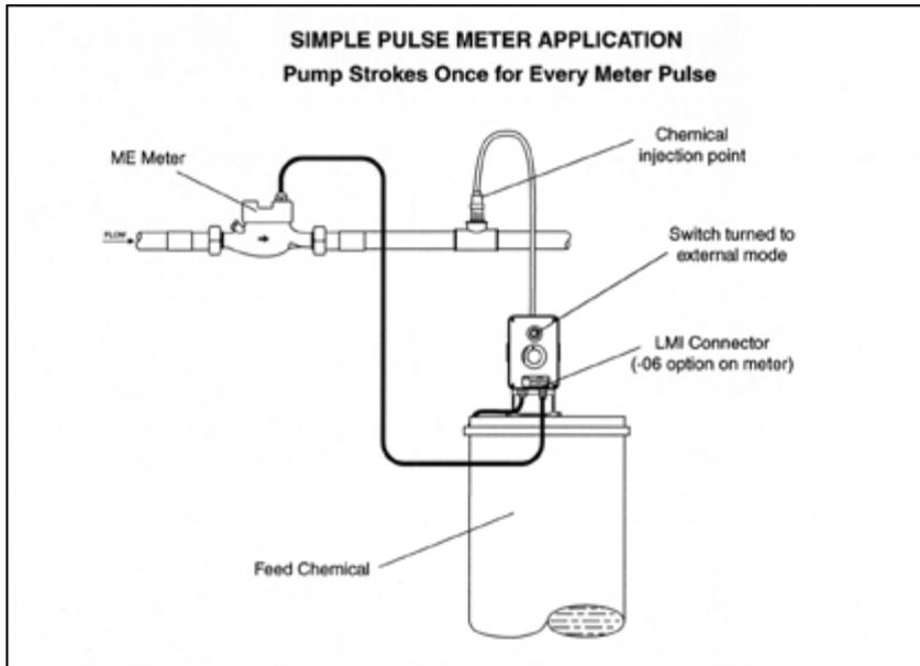
Use of a flow meter to control a metering pump is called “flow pacing” or “flow proportional feeding”. The main flow (usually of water) is monitored by the flow meter, which in turn controls a metering pump. In this way a chemical can be injected at a rate which matches the flow, for uniform concentration. Flow pacing can be done in one of four ways:
