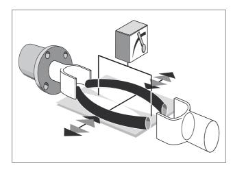
The mass flow alters the phase angle of the vibration, which produces a phase difference between the vibration at the tube inlet and that at the tube outlet. This phase difference is proportional to the mass rate of flow; it is amplified to form the output signal.
