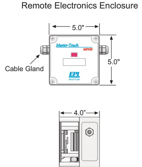
Two-wire, twisted pair interconnect cable required between Remote Electronics and Flow Transmitter (max. 5 ohm resistance).
