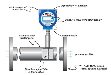
INLINE style thermal Flow Averaging Tubes have a flow section that is usually specified to match the user's flow conduit. It is plumbed directly into the process line. The standard design includes ANSI 150 # flanges and our flow straightening plates. Upstream straight run requirements can be reduced to a little as three diameters with this design. Our Inline style Flow Averaging Tubes are available in sizes from 2" pipe through 6" pipe (consult factory for larger sizes).
