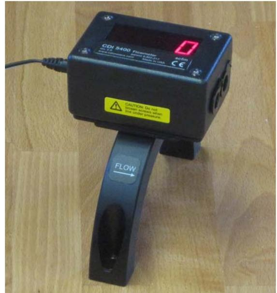
The CDI 5400 clamps onto a pipe, with two flow-sensing probes projecting into the pipe through 3/16-in. drilled holes. It seals directly to the pipe; no cutting or welding is required for installation. Because each flowmeter is made and calibrated for a specific size of pipe, the digital display indicates flow directly, with no setup or adjustment.
